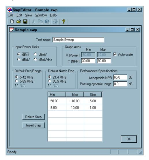
The table defines the steps used in the power sweep. The NprGraph program will process each segment definition line in turn by starting at the minimum power level, and repeatedly adding the step increment until the maximum level is reached. An NPR measurement is made at each step.
