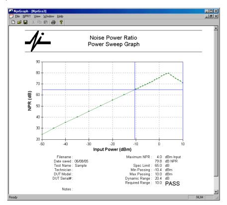
The graph plots measured NPR by Input Power. The data points are shown as dots connected by green lines. The header information is printed below the graph. The maximum NPR and the input power that produced the maximum are listed.
