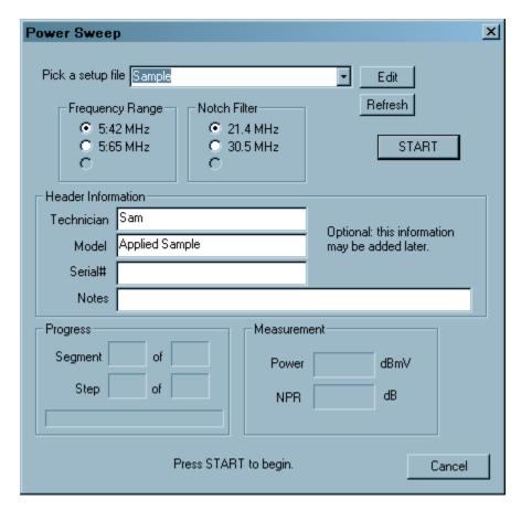
As the test is running, the progress will be shown in terms of segments and steps and the measurements will be displayed as they are obtained. At the same time, the graph will be drawn on the window behind the Power Sweep dialog box.
