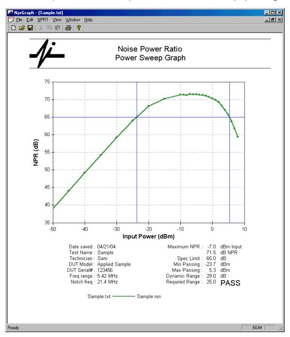
The graph includes a horizontal line at a specified NPR limit and calculates the points where the curve crosses the line. The difference between these two points is the usable dynamic range of the DUT and is compared to required range limit to determine a PASS/FAIL grade for the test.
